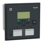
PowerLogic P3U20, 4L ringlug, 1U, 10DI/5DO, Uaux: 48-230V, DI: 220-230V, 2 x RJ-45
