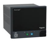
Protection and control relay, PowerLogic P7, transformer standard, 11CT, 7VT, 24BI, 20BO, 48-125V, ethernet RJ45
